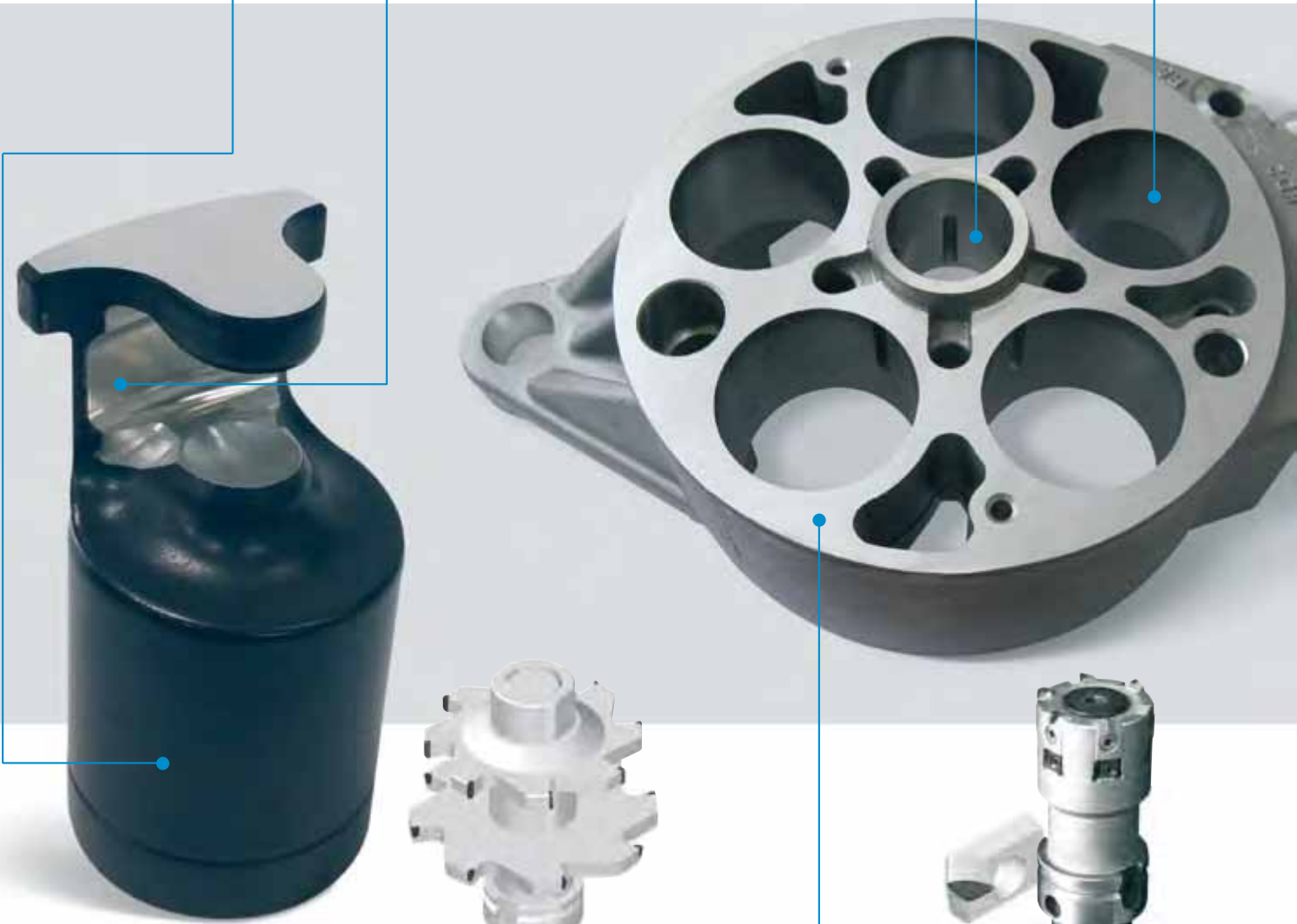
PCD milling cutter Piston housing face milling
