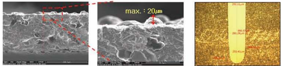
[Conventional Blade Surface and edge shape deformation]
