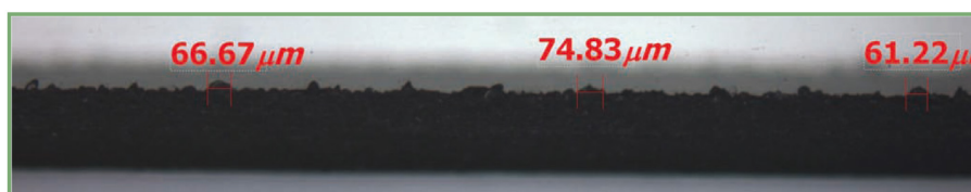
◆ Image of chamfered surface after using Metal #500
