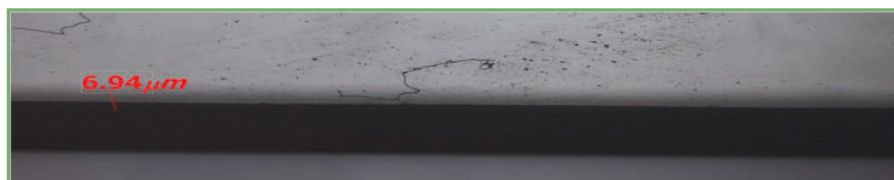
◆ Image of chamfered surface after using EHWA polyurethane wheel
